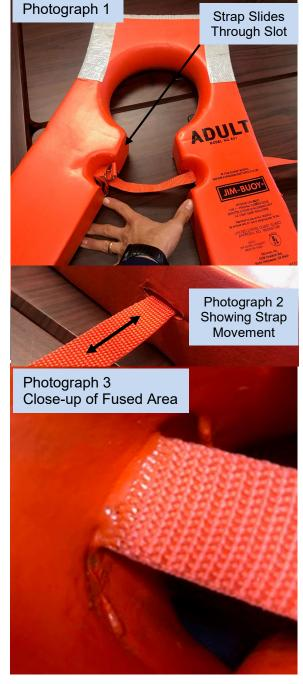
Because the cause of this defect could not be determined, the Coast Guard **strongly recommends** that Owners and Operators that have this type of PFD onboard their vessels inspect each one for this condition.
